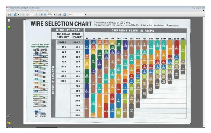
As a boat owner, you often have to be your own handyman as well. When installing wiring for new items, or replacing wiring for old ones, it is best to consult a wiring chart before you purchase the wire. Most situations can tolerate a 10% voltage drop, but not always. The chart here includes info on wire sizing factoring in a 3% voltage drop, instead of the typical 10%. If none of this means anything to you, call your electrician friend before starting.
