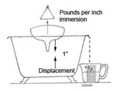
**Displacement:** If you weigh the boat on a scale, that is her actual (not advertised) displacement and the weight of sea water she will displace when afloat. Most designers figure displacement when half loaded (the boat, that is, not the designer) with stores, liquids, and crew.
